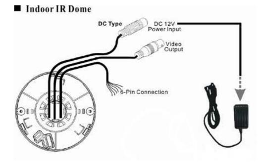
Connect the outdoor dome video output to a 75 Ohms type coaxial cable and the DC-Jack or AC/ DC-Terminator to the power source.
